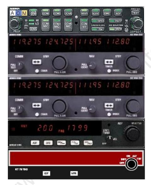
In order to standardize our cockpit configuration as much as possible, the normal procedure shall be to use the VHF - COM 1 for ATC and VHF - COM 2 for company, ATIS, 121.5 etc.. Radio communications will normally be handled by the CM 2 on the ground and by the PNF [PM] in the air.
